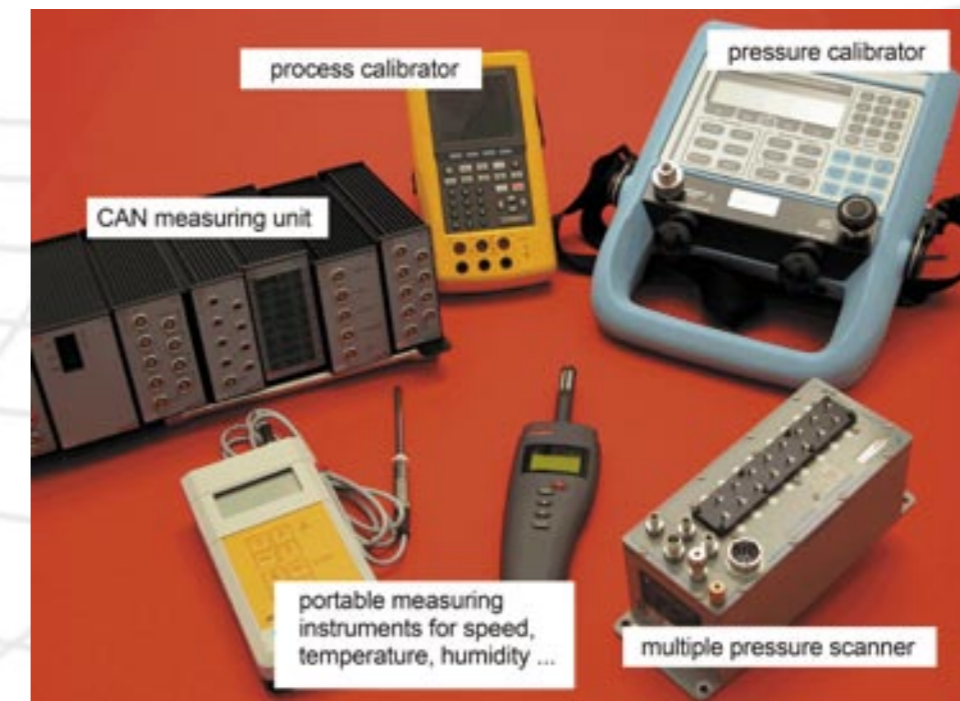
Fig. 25: Process and pressure calibrators.
