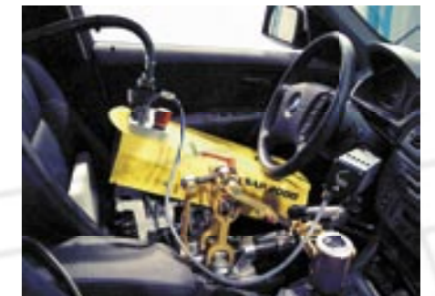
Fig. 12: The driving robot.
