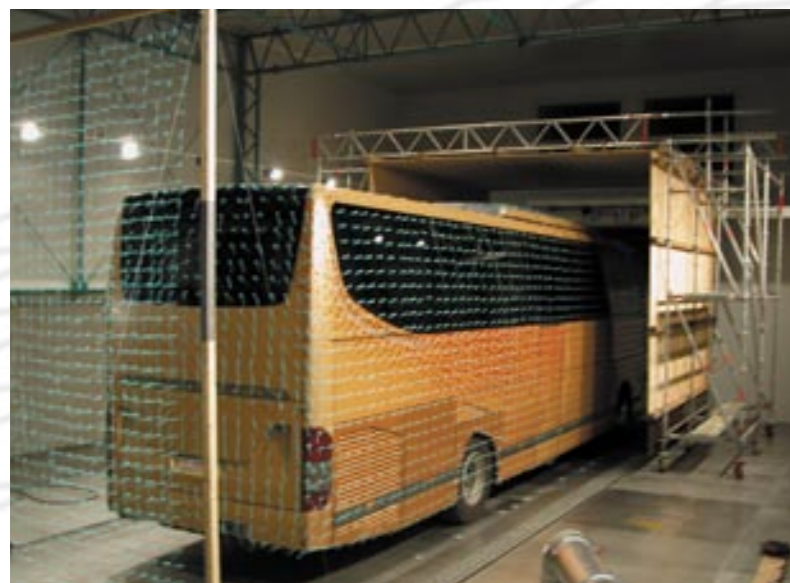
Fig. 8: A coach in the test section; the "mantel" improves the flow field around the sides and roof.
