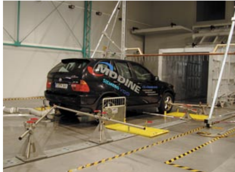
Fig. 6: A passenger car in the test section with the small nozzle.
