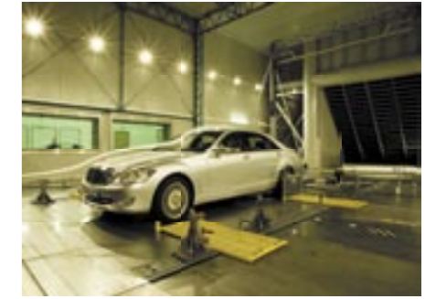
Fig. 9: The two-axle dynamometer.
