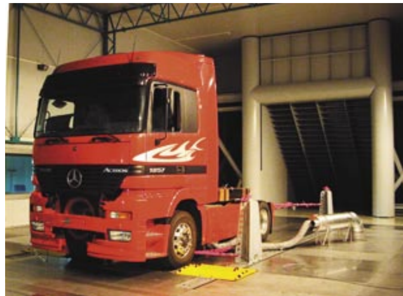
Fig. 7: A big truck in the test section, looking towards the collector.
