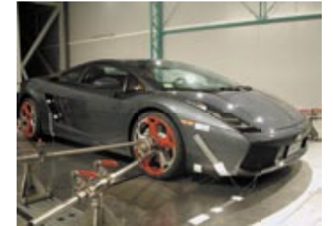
Fig. 10: Mountings for holding a passenger car on the dynamometer rollers.
