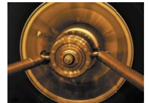
Fig. 11: Close-up of the rotating hub-adaptor.
